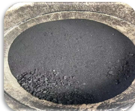
Sample of biochar produced: For further research studies in collaboration with NTU
